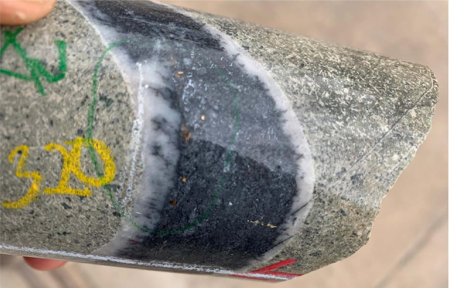
Photo 2: Drillhole MDDSC005 annotated HQ drill core (63.5 mm diameter) showing downhole depth and gold grades. Gold grades may slightly vary from those quoted in tables as laboratory assay repeats have been averaged during length weighted average calculations.
